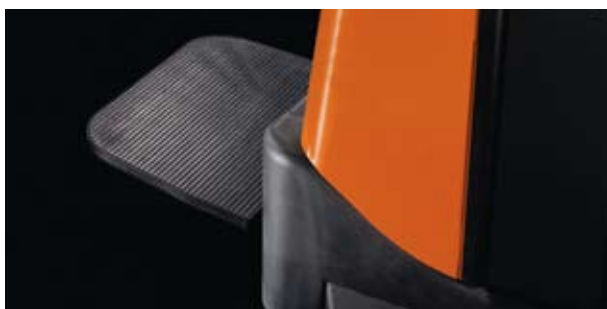
BT Levio P-series models' flip-down platforms aid productivity in long distance applications without compromising manoeuvrability
