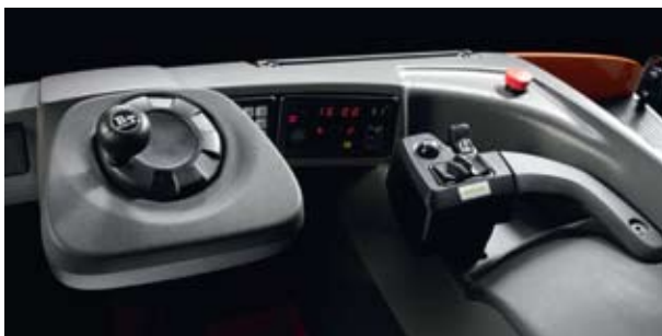
360° steering ensures maximum manoeuvrability and control with minimal effort
