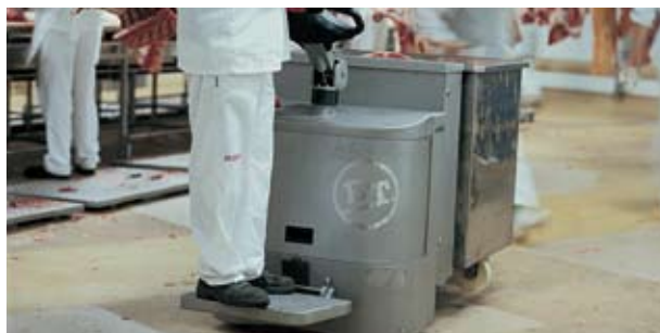
The LPE200I uses stainless steel for long-lasting performance in corrosive environments
