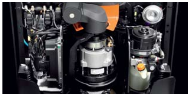
The fixed motor has no moving cables
